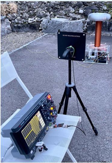
Fig. 12: The experimental setup of the voltage measurement via a measuring electrode.
