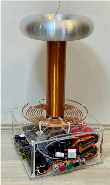
Fig. 3: An audio modulated DRSSTC with medium power output and characteristic toroidal top load.
